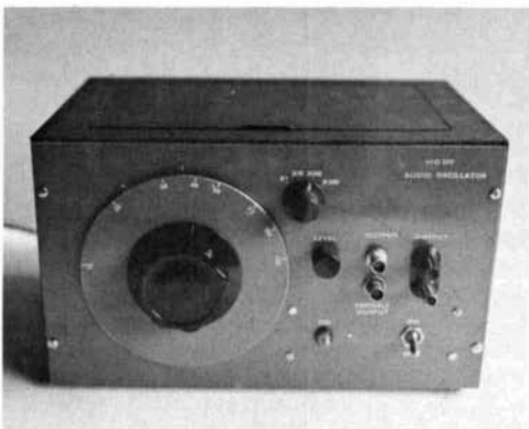
fig. 1. The original HO-200 audio oscillator used a tuning dial from an old HP-300 harmonic wave analyzer.
